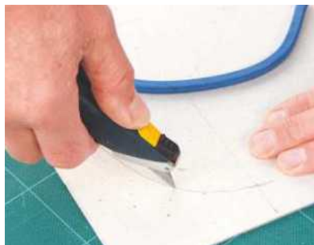
STEP 16. The shelf is supported by shaped brackets. A card template will help you get an even curve
